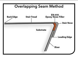
However, if the top edge of the riser extends up to or over the height of the step, trim riser to 1/4" - 1/2" from the top of the step to allow space for the EN-610 Epoxy Nose Filler Adhesive.
